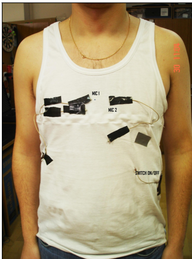
Fig. 3 The arrangement of the microphones and the on-off switch of the DVR
